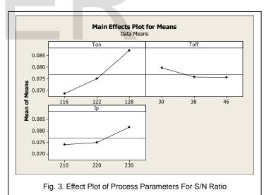
Fig. 3 above shows Mean Effective Plot for S/N ratios, which Clearly shows that input parameter level viz.  $T_{ON}$  -128,  $T_{OFF}$  - 30 and  $I_P$ -230 is having higher S/Nratio values.
