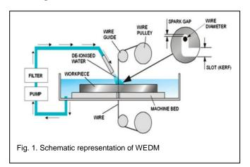
In this study, three important WEDM parameters, namely pulse-on-time (TON), pulse-off-time (TOFF) and peak current (IP) have been considered with three different levels each as shown in TABLE 2. Based on pilot experiments and literature survey the parameter range was selected. Other parameters
